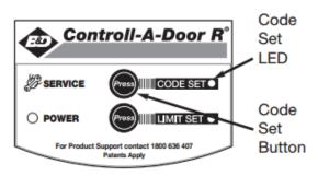
DIAGRAM 2 : ON OLDER STYLE DOOR MOTORS: THE CODE SET BUTTON IS SHOWN AS "2" IN DIAGRAM BELOW THE CODE SET LIGHT IS SHOWN AS "1" IN DIAGRAM BELOW
